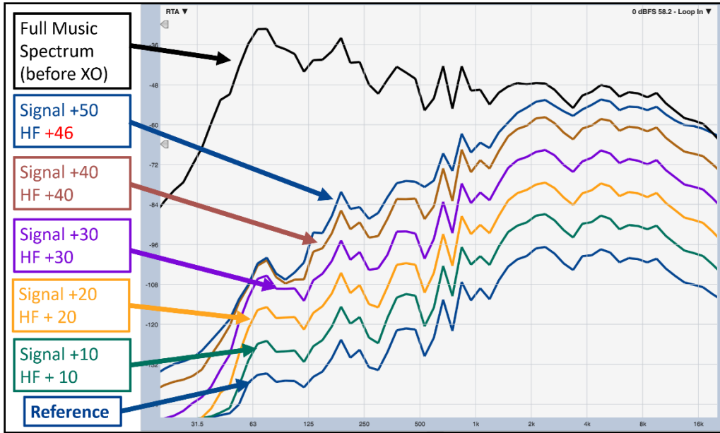
Figure 7 - Comparing level increase at the amplifier input ("Signal") to level increase at the HF crossover output ("HF")
